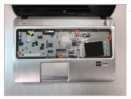
Using a Phillips #1 screwdriver, remove the four 5.6 mm silver screws.
