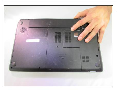
• Slide the release mechanism to the left to release the battery.
