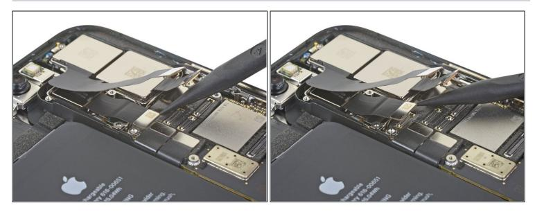
• Use a spudger to disconnect the third camera—its connector lies underneath the cable you disconnected in the previous step.
