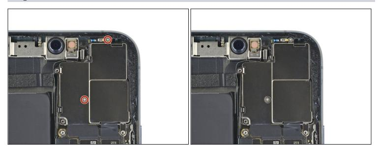
• Use a Y000 driver to remove the two 1.2 mm screws securing the rear camera cover.
