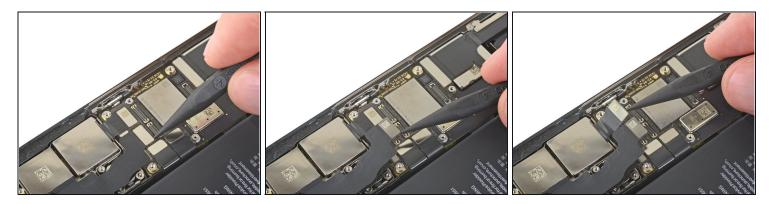
• Use a spudger or a fingernail to disconnect the first two camera cable connectors by prying them straight up from their sockets.
