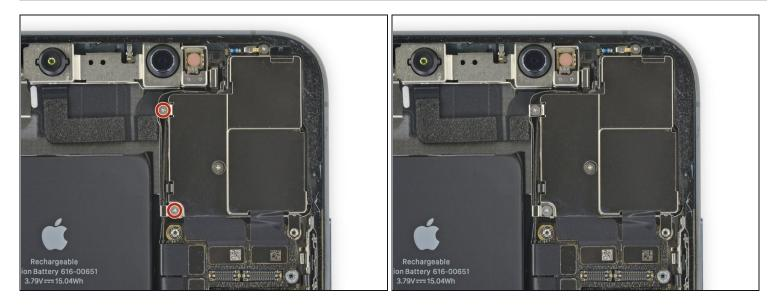
• Use a Y000 driver to remove the two 1.5 mm screws on the left side of the rear camera cover.
