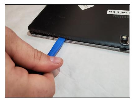
Remove the back cover with the blue plastic opening tool.
