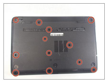
Using your Phillips #0 screwdriver, remove all of the screws on the back case.
