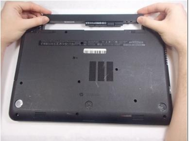
Press the tabs at the corners of the laptop at the same time to release the battery.
