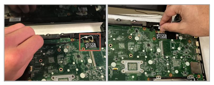
• Unclip the WLAN cable out of its place to allow the motherboard room to move.
