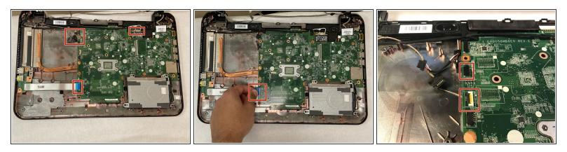
Disconnect the cables to the motherboard.
