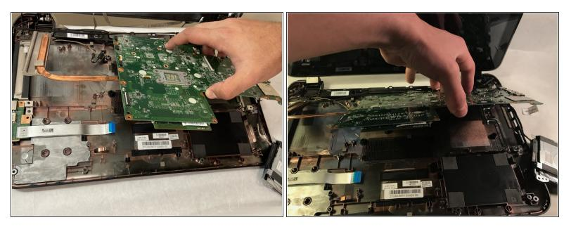
• Remove the motherboard from the device.
