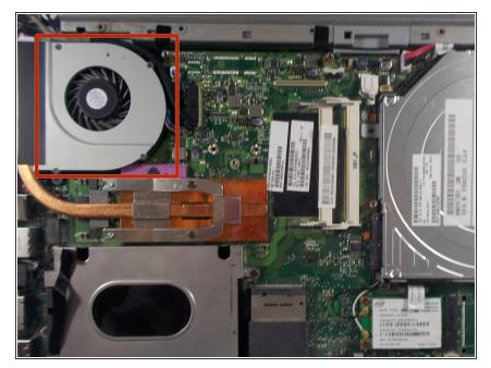
Locate the fan in the back left corner of the motherboard.
