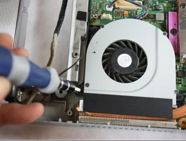
• Locate and remove the three Philips #00 5.65mm screws holding the fan in.
