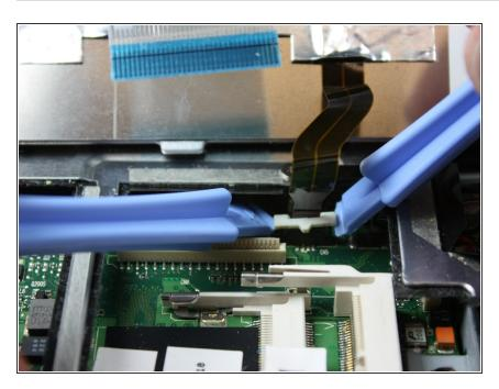
Using the plastic opening tools, pop out the second ribbon cable from the rest of the computer.
