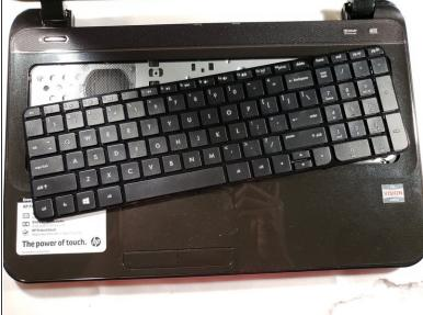
Using a plastic opening tool, release the keyboard clips.
