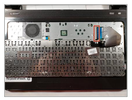
Tilt the keyboard to expose the Zero Insertion Force connector to which the keyboard cable is attached.
