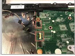
Disconnect the cables to the motherboard.
