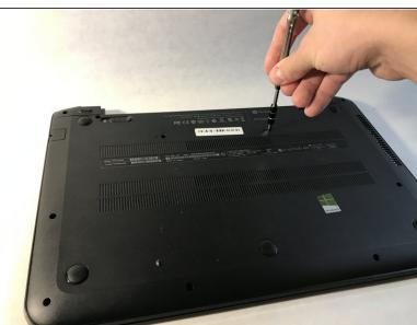
Use JIS #1 screwdriver to remove the eleven 6 mm screws.
