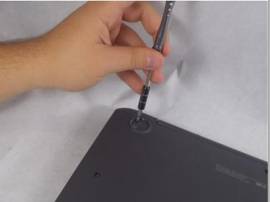
Remove the two 9mm Phillips #1 screws.
