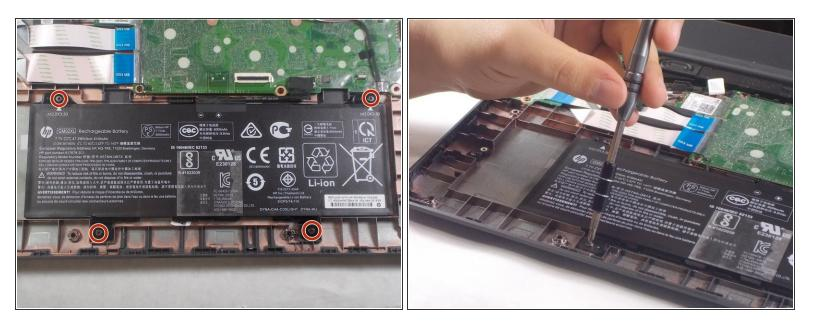
Remove the four 4mm Phillips #0 screws from the battery.
