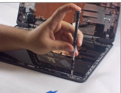
Remove the four 2mm JIS #000 screws.
