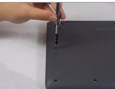
Remove the seven 6mm Phillips #00 screws found underneath the stoppers.
