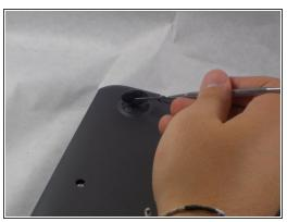
• Remove the two bigger rubber stoppers using a metal spudger.
