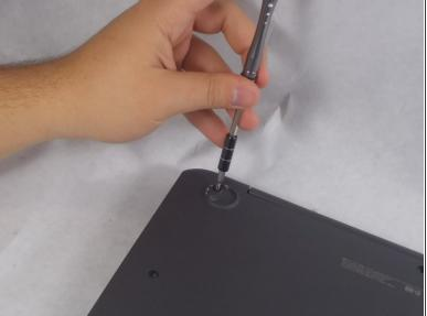
Remove the two 9mm Phillips #1 screws.
