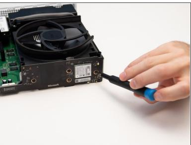
Remove the four 15mm screws attaching the IR Blaster to the metal chassis with the Torx T8 Security screwdriver.
