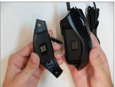
Remove the interchangeable side plate.
