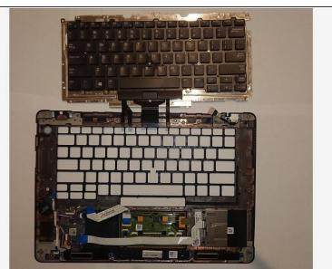
Disconnect the four ribbon wires labeled by the red rectangles by pushing aside the metal release tab and gently pulling the ribbon wire.
