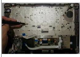
• Use a Phillips #0 screwdriver to remove the seventeen 4 mm screws.
