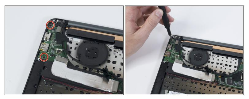
Use a Phillips #00 screwdriver to remove the two, 3mm screws from the USB-A and HDMI port module.
