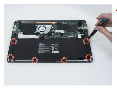
Use a Phillips #00 screwdriver to remove the six, 5mm screws securing the battery.
