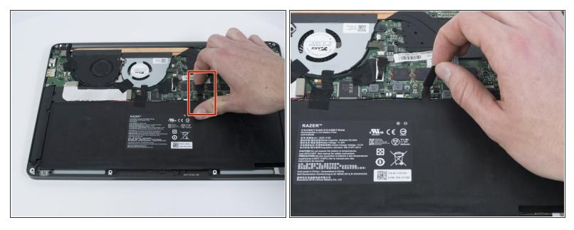
• Use your fingernail to pry up and disconnect the battery from the motherboard.
