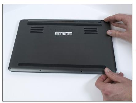
Remove the bottom cover of the laptop by sliding it away from the hinge.
