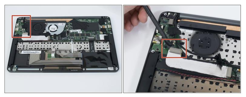
Use a plastic spudger to lift up the press-fit interconnect cable and expose the USB-A and HDMI port module.
