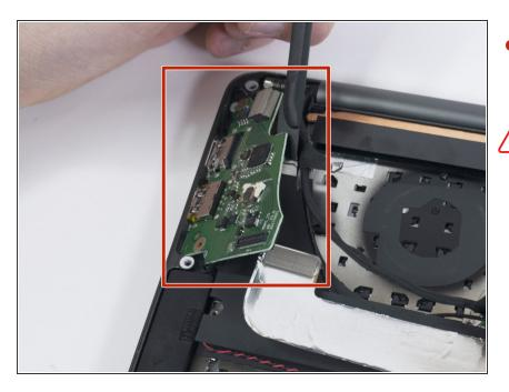
Use a plastic spudger to remove the USB-A and HDMI port module from the case.
