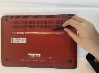
Remove twelve 7.5 mm screws by using the Phillips #00 screwdriver.
