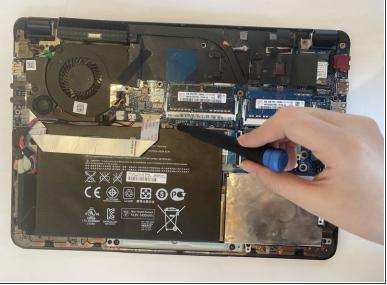
Remove three 4.2mm screws by using the Phillips #00 screwdriver.
