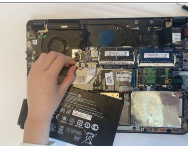
Disconnect the battery cable from the motherboard and remove the battery from the device.
