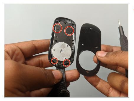
Remove the four screws using a Phillips #000 screwdriver.
