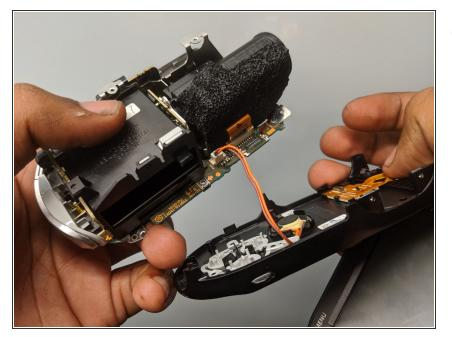
• Pull apart the sides of the camera once the screws are removed.
