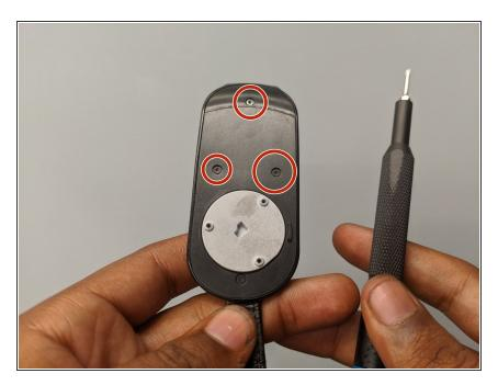
• Remove the three screws using the Phillips #000 screwdriver.
