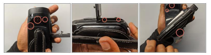
• Remove all eight screws using the Phillips #000 screwdriver.
