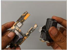
Remove the lens assembly from the device.
