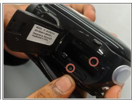
Unscrew the eight 4mm screws using the Phillips #000 screwdriver.
