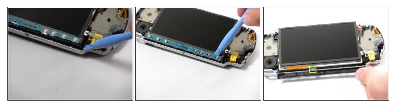
• Remove the home bar by gently prying on the left and right sides of it with the opening tools. Lift the bar out of the device.
