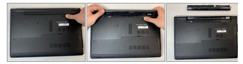
When the battery pops out, lift it so that it comes out completely.
