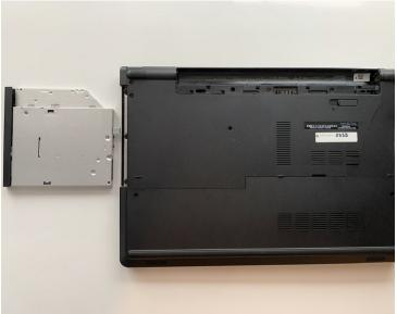
Pull the optical drive horizontally to the left to remove it from the laptop.
