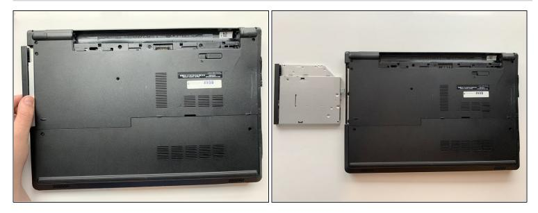
• Pull the optical drive horizontally to the left to remove it from the laptop.
