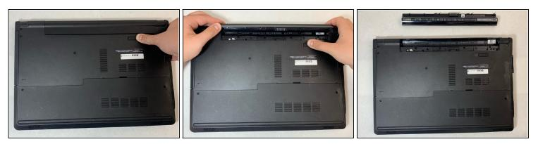
• When the battery pops out, lift it so that it comes out completely.
