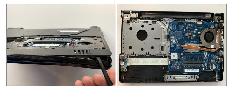
• Using the flat end of the spudger, pry the bottom base off of the laptop by the crack around the perimeter of the laptop and running the spudger around the edges.
