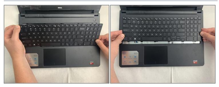
• Lift up and slide back to release the six notches from the bottom of the keyboard.
