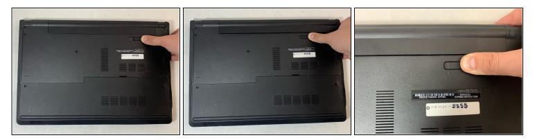
• Push the lock switch to the left to pop out the battery.
