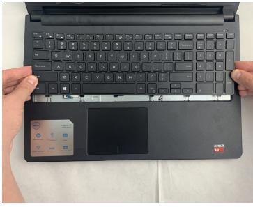
• Lift up and slide back to release the six notches from the bottom of the keyboard.
