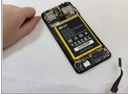
Remove the rubber protective covering from the side of the speaker using the <u>tweezers</u>.
