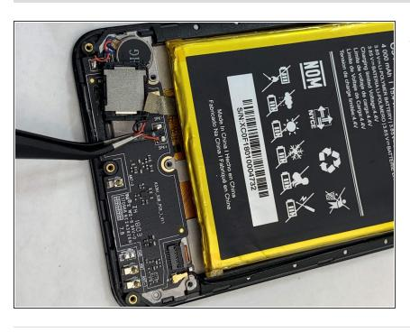
De-solder the wires from the bottom sub-frame and the speaker. Use the <u>link</u> listed to safely de-solder the speaker.
