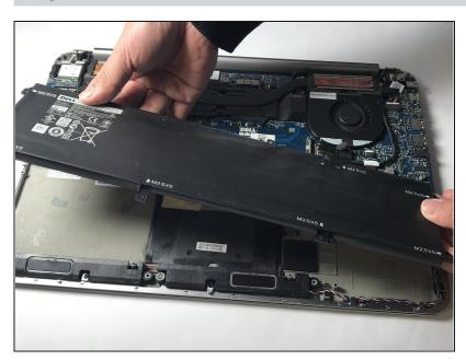
• Lift the battery off the chassis.
