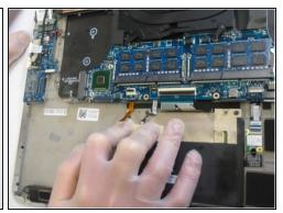
Using both hands and plastic tweezers, disconnect the cables from the laptop base.
