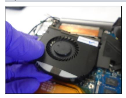
Remove the fans by gently lifting up the edges until the fans disconnect from the motherboard completely.
