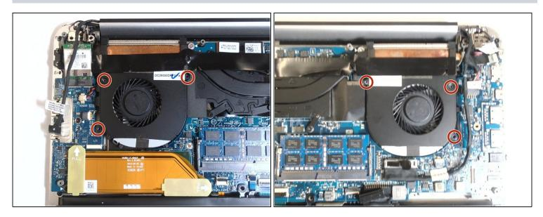
Use the Phillips #0 screwdriver to unscrew the three screws on each fan.
