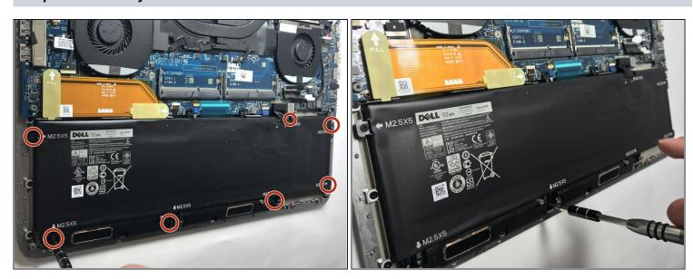
Using a Phillips #0 screwdriver, remove the seven 3.5mm screws that secure the battery to the palm rest assembly.
