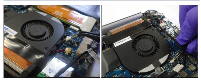
Use metal tweezers to carefully unplug the fan cables from the motherboard.
