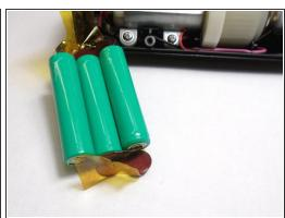
Carefully peel the tape off far enough to remove the 3 batteries.
