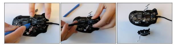
• Using the opening tool, pry the black bracket holding the scroll wheel in place backwards until the scroll wheel housing pops out.
