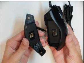
• Remove the interchangeable side plate.
