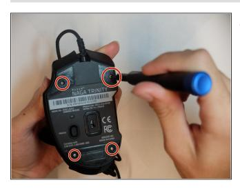
Remove the four 6mm screws by using a JIS #1 screwdriver.
