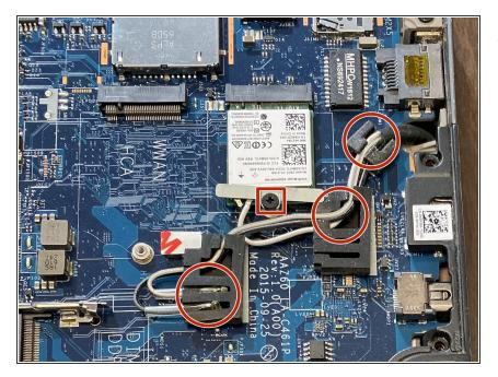
Remove wires in protectors (red circles) and remove the screw in red square. Pick the wires out of the motherboard.
