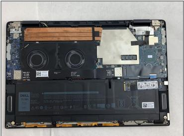
• Carefully slide the SSD from its port, removing it from the device.
