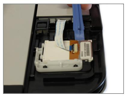
After removing the top cover of the LCD assembly, remove the LCD using the plastic opening tool.
