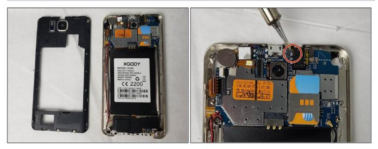
• Use the soldering iron and <u>desoldering pump</u> to remove the six soldered connections that are holding the headphone jack to the motherboard.
