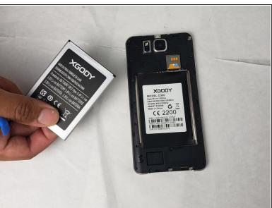
Remove the battery using your hands or the plastic opening tool.
