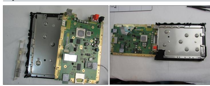
• Once the heatsink is removed, cautiously pull the motherboard out from the left side of the console case and remove it from the device.
