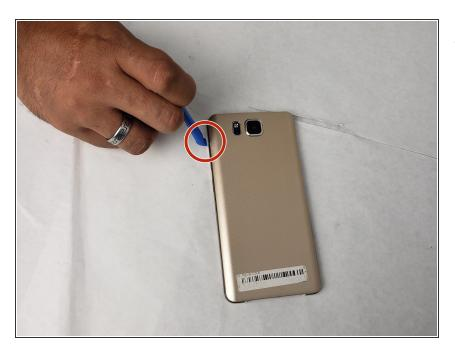
Insert the pry tool into the seam and pry the back cover of the case along the seam until the cover is free of the case.
