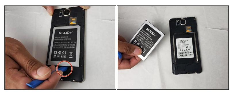
Remove the battery using your hands or the plastic opening tool.
