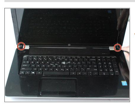
Using a Phillips #0 screwdriver, remove the two 5 mm screws in the lower left and right-hand corner of the laptop screen.
