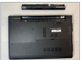
When the battery pops out, lift it so that it comes out completely.
