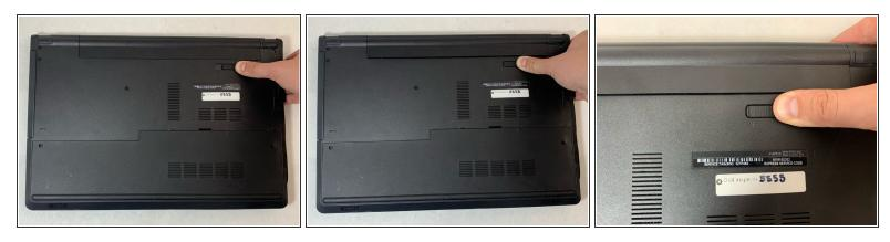
Push the lock switch to the left to pop out the battery.
