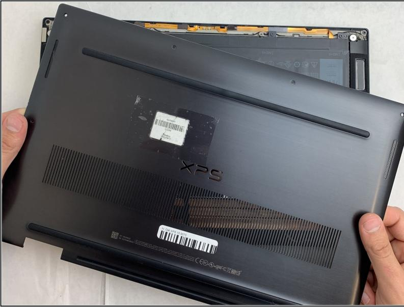
**⚠** Make sure all screws are removed before you lift the panel to prevent any damage from occurring.
