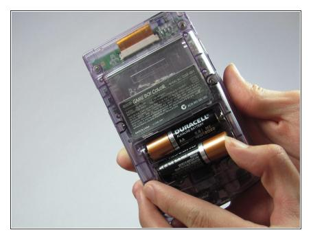
Remove the batteries from the battery compartment.
