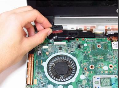
• Use the tip of the blue plastic opening tool to gently flip-up the black locking flap of the cable connecting the motherboard to the display.
