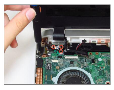
Remove all of the screws from the black hinge mounts on either side of the device using a Phillips #00 screwdriver.
