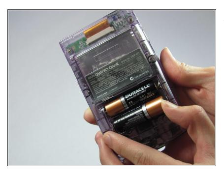
Remove the batteries from the battery compartment.
