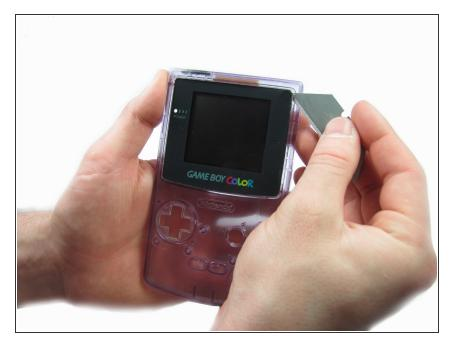
Carefully slide a razor blade under one of the corners of the screen cover.
