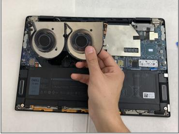
• The fan has been completely disconnected and is now safe to remove.
