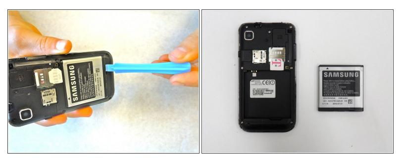
Remove the battery by pushing the bottom edge of the battery up and away from the phone
