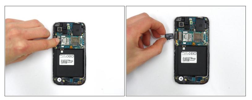
Slide the SD card out of its slot.
