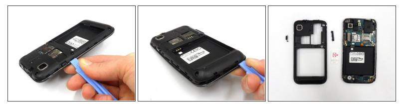
• Staring near the power button, use a plastic opening tool to disengage the plastic clips securing the midframe.
