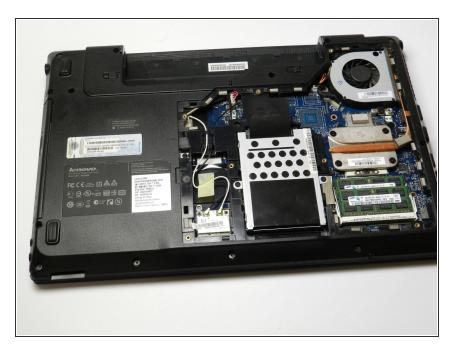
The computer should be open with many of the internal components shown. You can now access the hard drive, the RAM, and the keyboard.
