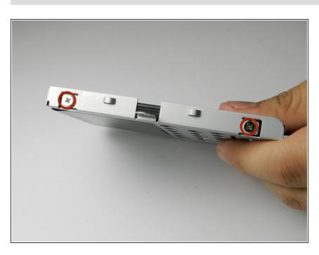
Unscrew the four 5.2 mm Phillips #1 screws. There are two on each side of the drive holding it in the drive bay.
