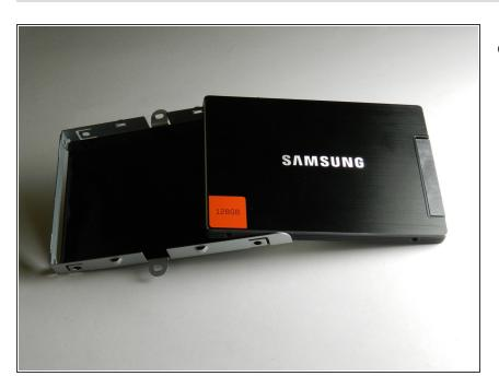
Pull the drive out of the bay. If all the screws were removed correctly, it should simply slide out.
