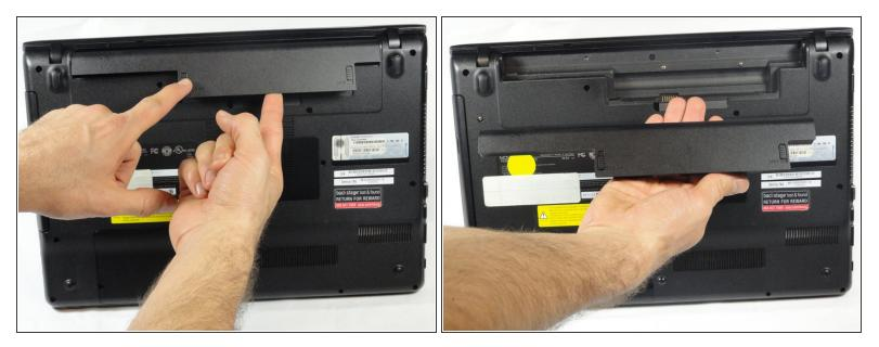
• Remove the battery out from the notch while continuing to hold the release button.
