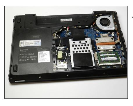
The computer should be open with many of the internal components shown. You can now access the hard drive, the RAM, and the keyboard. To reassemble your device, follow these instructions in reverse order.
