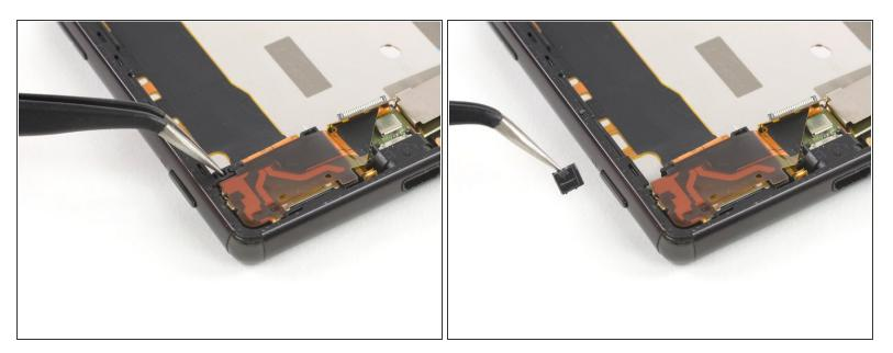
Also remove the plastic safeguard between the midframe and the loudspeaker cover.
