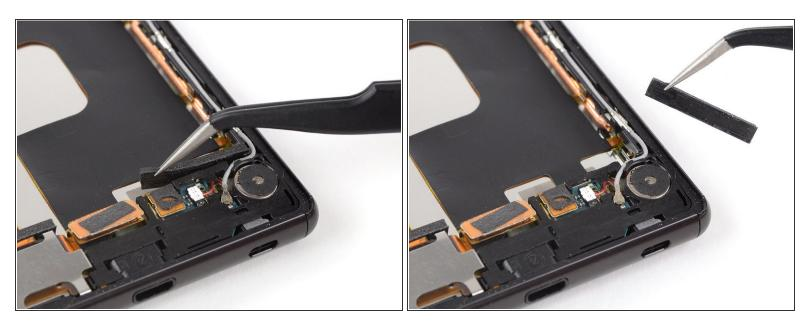
Use a pair of tweezers to peel off and remove the foam pad on top of the daughterboard.
