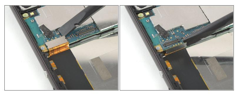
Use a spudger to pry up and disconnect the side button flex cable on the left side of the motherboard.
