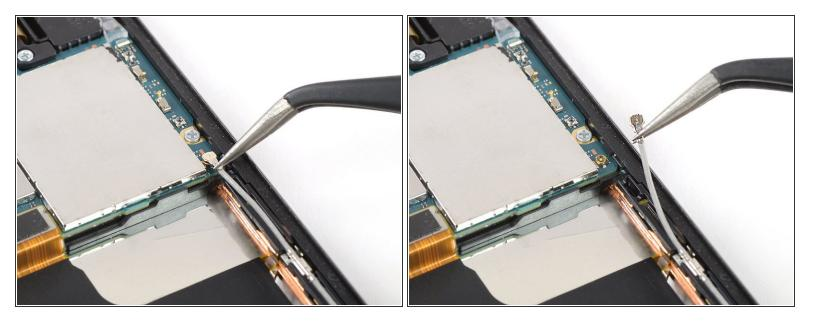
Use a pair of tweezers to pry up and disconnect the upper connector of the antenna cable.
