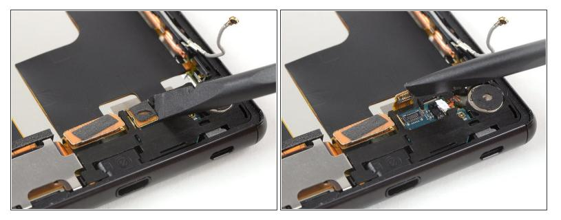
Use the flat end of a spudger to pry up and disconnect the small main flex connector next to the vibration motor connector.
