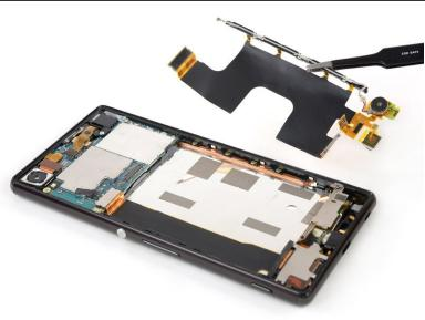
Use a pair of tweezers to remove the main flex cable assembly including the vibration motor and the microphone.
