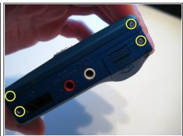
Start by removing the 8 very small screws on both sides of the unit. The front door will still be connected via the latch.
