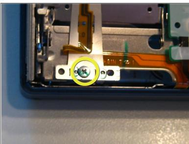
■ The front panel may now be removed. Next, remove one screw on the inside front panel.
