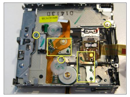
Remove the remaining 10 visible screws which connect the laser eye and related mechanism. Start from the bottom up as they will release various latches and connectors from the unit.
