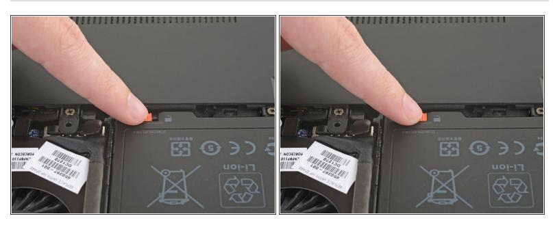
Slide the switch with the padlock symbol toward the unlocked side.
