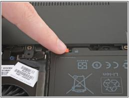
To install your new battery, press it into place so that it lays flat, then slide the red switch with the padlock symbol back to the **locked** side.
