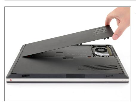
Lift up and remove the battery cover.
