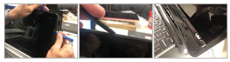
• Using two plastic removal tools or a spudger, gently work around the LCD bezel until it is free from the LCD case. Apply heat as necessary, however, use caution as heat can warp the bezel.
