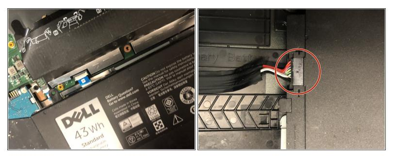
Disconnect the Battery from the mainboard to ensure power is not running through the board during the repair.
