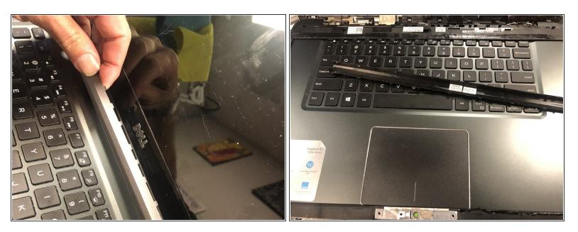
Remove the plastic bracket that sits between the LCD and the keyboard.
