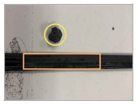
Clean off all old adhesive from the LCD bezel. Roll the adhesive into a ball and discard.
