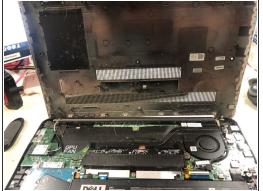
Remove the clamshell from the top down using a smudging tool. The shell should come off fairly easily without much resistance.
