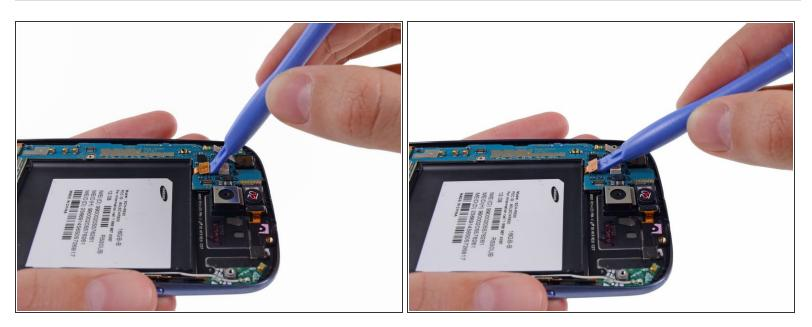
• Disconnect the digitizer cable by gently prying its connector up from its socket on the motherboard.
