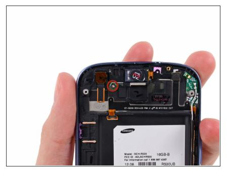
Remove the single 2.0 mm Phillips screw securing the front-facing camera bracket to the front panel.
