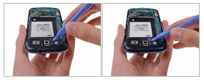
Use a plastic opening tool to pry the rear-facing camera connector up from its socket on the motherboard.
