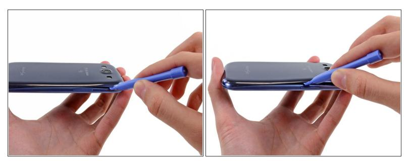
Continue to move the plastic opening tool around the perimeter of the top left corner, gently prying up along the rear case.
