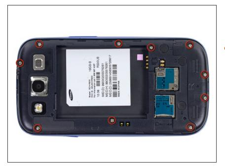
Remove the ten 4.0 mm Phillips screws securing the midframe to the front panel assembly.
