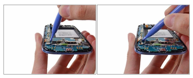
• Disconnect the display data cable from the motherboard.
