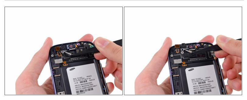
• Use a pair of tweezers to lift the front-facing camera/ambient light sensor/rear microphone assembly out from its socket in the front panel assembly.
