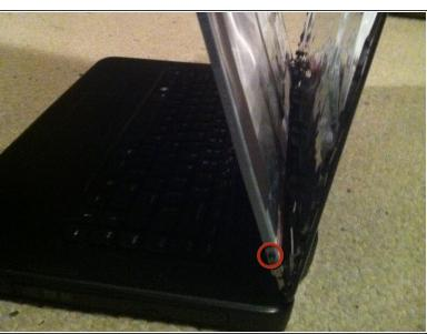
Now remove the four screws that hold the screen in the metal frame. There are two on each side
