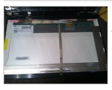
Once all the screws have been removed and the camera cable disconnected you can lay the screen down on your keyboard to disconnect the other cable.
